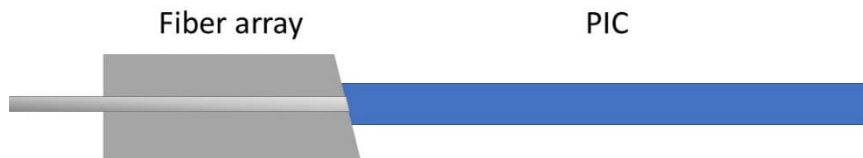
Figure 15: Angled polishing of the fiber-to-chip interface
