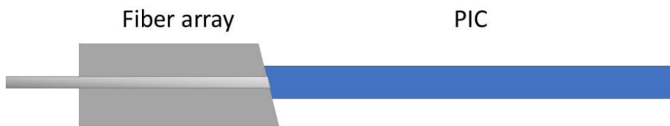
Figure 17: Angular polishing of the fiber-to-chip interface
