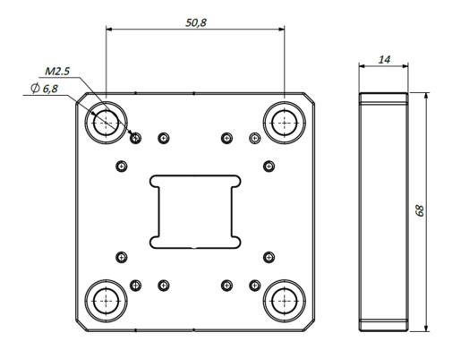
Figure 1: PHIX Cooling Carrier mounting base dimensions
